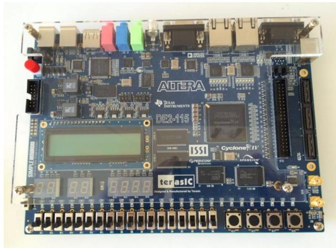
Fig.5. Altera DE2-115 FPGA board
