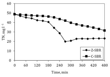
Fig. 5. Variation of TN profiles in C-SBR and Z-SBR.
