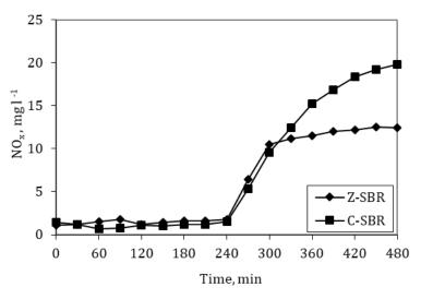
Fig. 4. Variation of  $NO_x$  profiles in C-SBR and Z-SBR.
