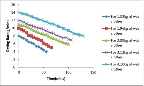
Fig. 3. The variation of drying rate with time
