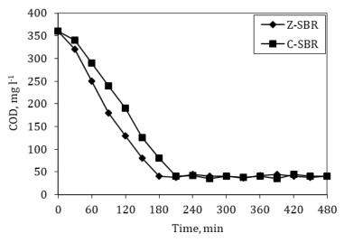
Fig. 2. Variation of COD profiles in C-SBR and Z-SBR.
