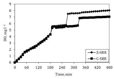
Fig. 7. Variation of DO profiles in C-SBR and Z-SBR.
