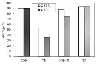
Fig. 1. Pollutant removal performance of C-SBR and Z-SBR.
