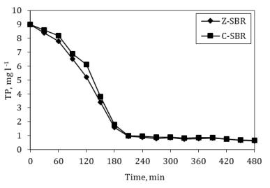
Fig. 6. Variation of TP profiles in C-SBR and Z-SBR
