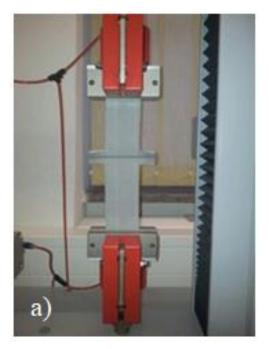
Figure 2. Experimental device for unidirectional texting
