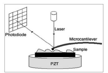
Figure 5. A schematic diagram of AFM (Balthazar et al., 2013).
