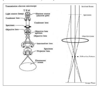
Figure 2. The layout of optical components in a basic TEM (Williams and Carter, 2009).
