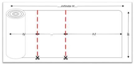
Figure 1. First stage of guillotine cut
