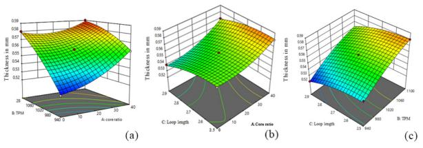
Figure 5. Thickness of knitted fabrics produced from cotton/polyester core spun yarns
