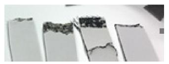
Figure 3. The samples subjected to tensile force during the adhesion test
