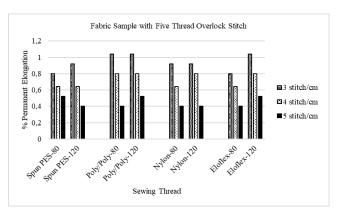
Figure 16. Permanent elongation values (after 2 hours) of the fabric sample with five thread overlock stitch
