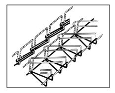
Figure 6. Stitch type 516 (Five thread overlock stitch) [14]
