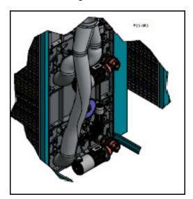
Figure 4. Dedusting System (Brush Vacuumed System)
