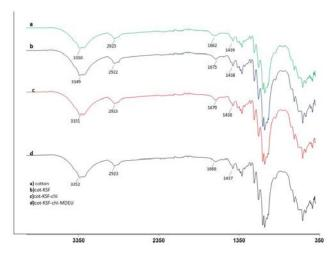
Figure 1. FTIR Analysis of untreated cotton, cot-KSF, cot-KSFchi, and cot-KSF-chi-MDEU.
