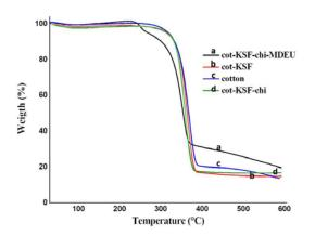
Figure 3.TG curves of samples untreated cotton (c), cot-KSF (b), cot-KSF-chi (d), and cot-KSF-chi-MDEU (a).
