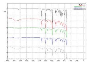
Figure 2. FT-IR spectrum for VIM and PVIM samples
