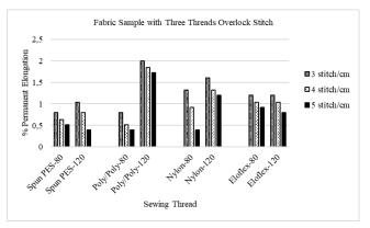
Figure 14. Permanent elongation values (after 2 hours) of the fabric sample with three thread overlok stitch
