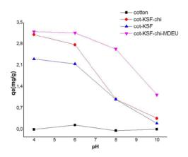
Figure 4. Impact of pH on dye adsorption of cotton, Cot- KSF, Cot- KSF -chi, and Cot- KSF -chi-MDEU.
