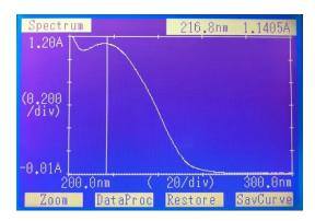
Figure 5. UV-visible spectrum of PVIM in H<sub>2</sub>O solution
