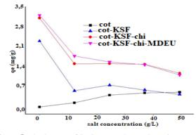
Figure 5. The impact of ionic strength on adsorption capacity of cotton, Cot- KSF, Cot- KSF -chi, and Cot- KSF -chi-MDEU.
