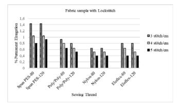
Figure 8. Permanent elongation values (after 2 hours) of the fabric with lockstitch
