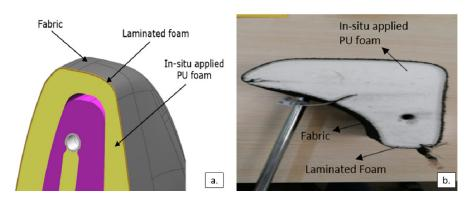
Figure 2. Headrest components a. Schematic image of headrest b. Real image of headrest
