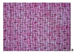
Figure 7. Surface images of W-1 A) Untreated B) 50 g/l PVIM treated
