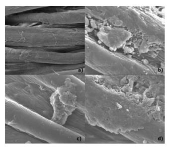
Figure 2. SEM figure of a) untreated cotton, b) cot-KSF, c) cot-KSF-chi, and d) cot-KSF-chi-MDEU.
