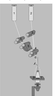
Figure 2. Core spinning process diagram 1. Cotton roving,
