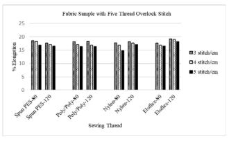
Figure 15. Elongation values (after 30 minutes) of the fabric sample with five thread overlock stitch
