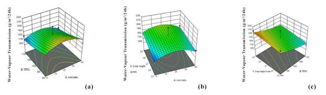
Figure 7. Water-vapour transmission of knitted fabrics produced from cotton/polyester core spun yarns
