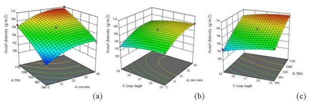
Figure 4. Areal density of knitted fabrics produced from cotton/polyester core spun yarns
