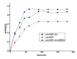
Figure 6. The impact of contact time on adsorption.
