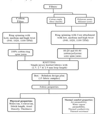
Figure 1. Experimental plan
