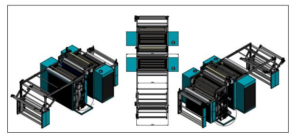
Figure 8. Design and Production of Raising Machine
