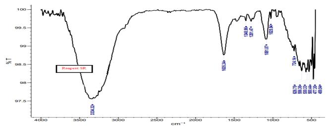
Figure 2. FT-IR analysis of the commercial finishing agent (Reapret SR)
