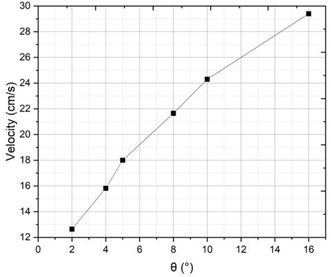
**Figure 5.** Variation of water flow velocity with respect to suspension arm deviation angle  $\theta$
