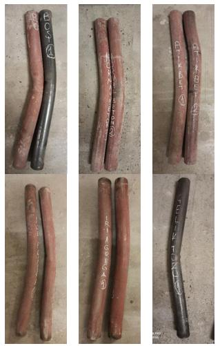
**Figure 5.** Test specimens after buckling
