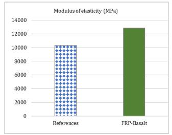
**Figure 6.** Graphs of modulus of elasticity of beams reinforced with reference and basalt-based FRP polymer
