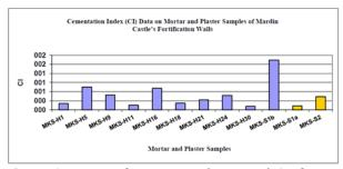
**Figure 14.** X-Ray Fluorescence (PED-XRF) Analysis Cementation Index Data on Mortars
