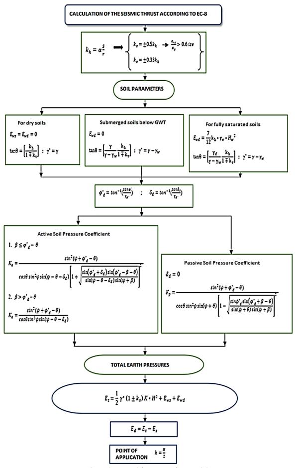
Figure 2. Design Schema according to EC-8
