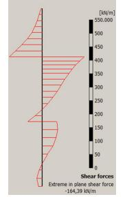
Figure 14. Maximum plane shear force
