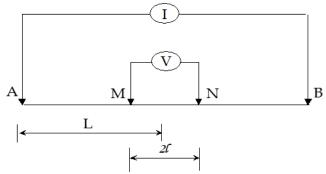
Figure 1. Schlumberger Electrode Configuration.
