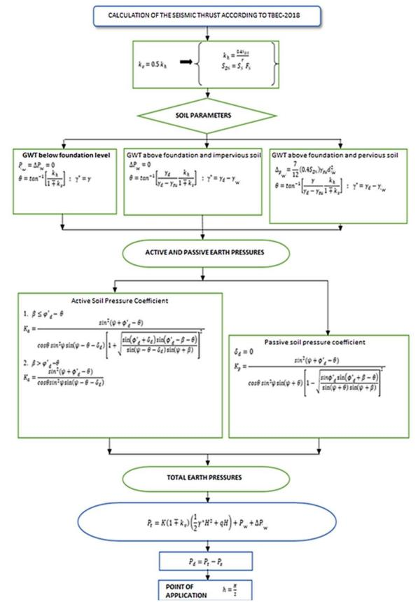
Figure 1. Design Schema according to TBEC-2018
