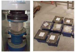
Figure 2. Cubic concrete specimens and compressive test
