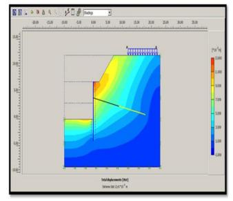
Figure 16. Total Lateral displacement
