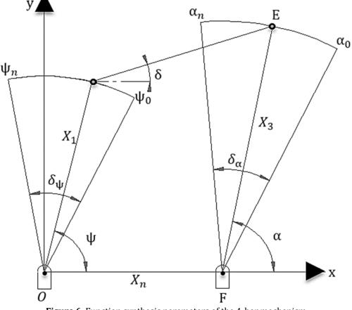
Figure 6. Function synthesis parameters of the 4-bar mechanism
