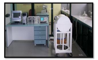
Figure 7. Canberra GC 1519 model HPGe detector
