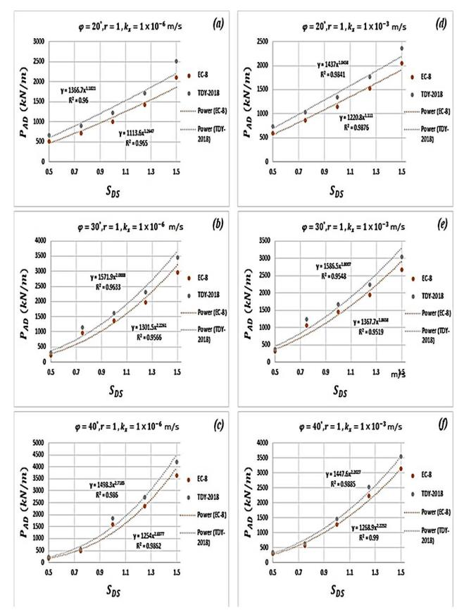
Figure 4. Variation of horizontal dynamic active thrust forces acting on the anchored wall with earthquake acceleration coefficient
