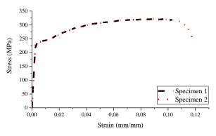
Figure 3. Tensile test results for the steel tube
