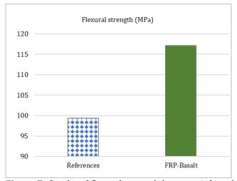
**Figure 7.** Graphs of flexural strength beams reinforced with reference and basalt-based FRP polymer
