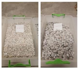
Figure 1. 1-4 mm (fine) and 4-16 mm (coarse) aggregate
