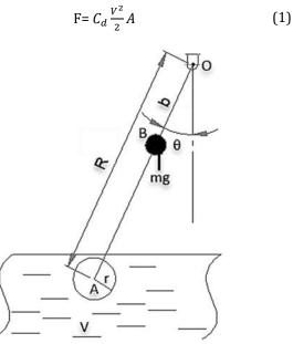
**Figure 4.** A device for measuring the water flow rate in an open channel
