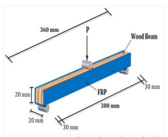
**Figure 3.** Sample prepared according to the standard for bending test
