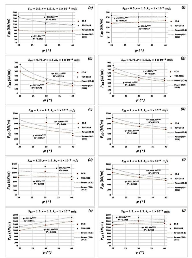
**Figure 7**. Variation of horizontal dynamic active thrust forces acting on the yielding gravity wall with the internal friction angle of the soil ( $\phi_d$ ) according to EC-8 and TBEC-2018 Regulations
