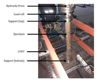
Figure 4. Test setup and instrumentation
