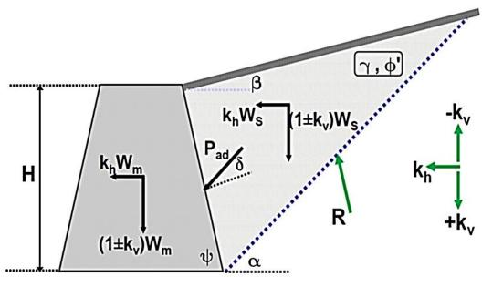
Figure 3. A simplified drawing for the gravity retaining wall (Eurocode-8)
