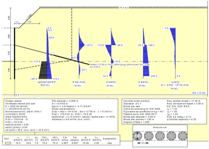
Figure 4. GGU-Retain analysis results of the model
