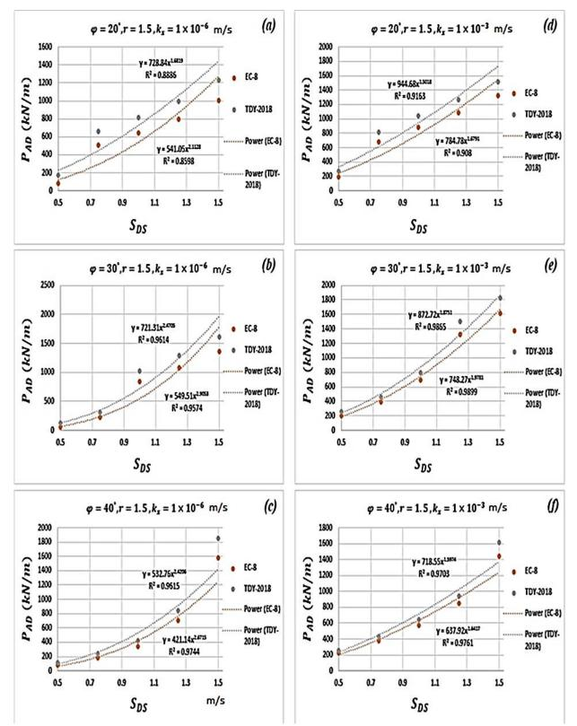
**Figure 5.** Variation of horizontal dynamic active thrust forces acting on the yielding gravity with the earthquake acceleration coefficient
