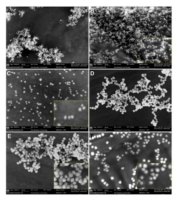
**Fig. 1.** SEM images of synthesized gold nanoparticles. (A) AuNP20. (B) AuNP<sub>23</sub>-PEI. (C) AuNP<sub>24</sub>-PEG. (D) AuNP<sub>50</sub>. (E) AuNP<sub>56</sub>-PEI. and (F) AuNP<sub>57</sub>-PEG. AuNP = gold nanoparticles, PEI = polyethyleneimine, PEG = polyethylene glycol.
