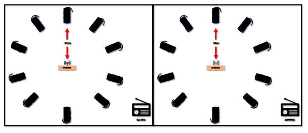
Fig. 1. The experimental setup for the exposure of 900 and 2100 MHz RFR.
