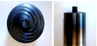
**Figure 7.** Tool with hollow spherical shoulder and cylindrical threaded pin [23]
