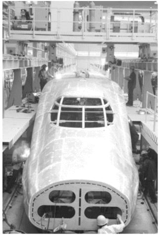
**Figure 15.** FSW robot system for high speed trains [68]
