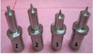
Figure 3. Examples of tools with different pin geometries [21]
