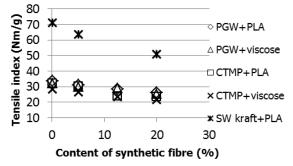
Figure 2. Tensile index of the sheets as a function of the synthetic fibre content. With PGW and CTMP the standard deviation ranged from 0.8 to 2.2 Nm  $g^{-1}$  and in SW kraft from 2.0 to 2.8 Nm  $g^{-1}$  (Asikainen & Korpela 2014)
