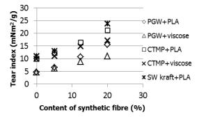
Figure 1. Tear index of the sheets made with a minor share of synthetic fibre. With PLA the tear index increased 117% in CTMP and 243% in PGW stock, while with the viscose fibre the index increased 77% and 141% respectively. In softwood kraft the tear index increased 118% (Asikainen & Korpela 2014)
