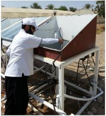
Figure 1. Four solar stills at the Experimental Station of Sultan Qaboos University.
