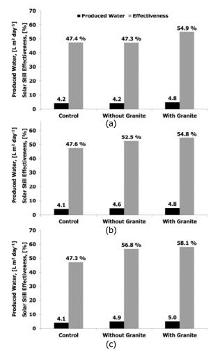
Figure 2. Water production and solar still effectiveness of three solar stills; conventional (control), without and with granite solar absorbers under three treatments; (a) no cover cooling, (b) low flowrate and (c) high flowrate of cold water cooling.
