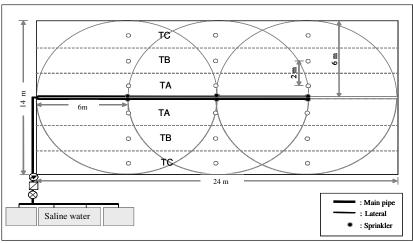
Figure 1. Layout of the experiments under rain-shelter
