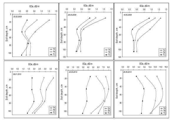
Figure 2. Soil salinity builds up in the rain shelter
