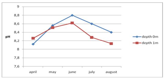
Figure 2. Water pH in the Zhrebchevo Dam Lake at 0 m and 1 m depth
