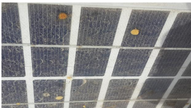
Fig. 2. Dust deposited on a PV module
