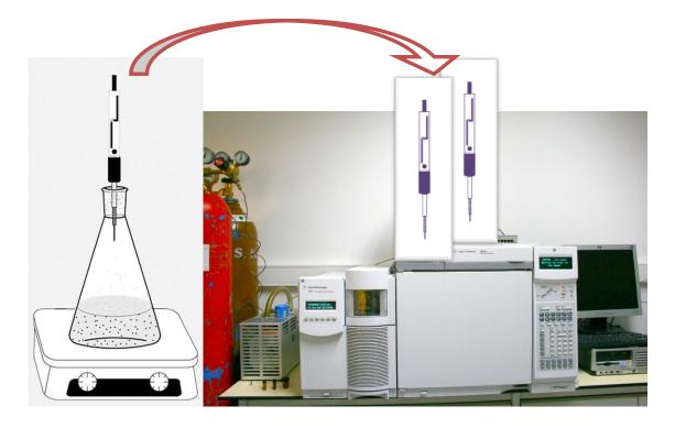
Figure 2. Analysis of the volatiles by using HS-SPME/GCMS technique
