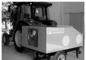
Figure 1. Tractor PTO test system.
