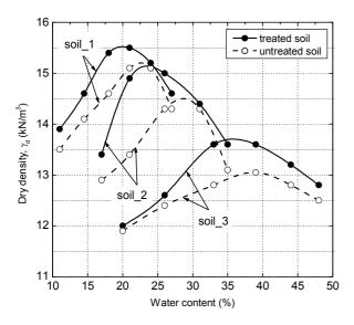
Figure 1. Water content-dry density relationship for the three soil types, both treated and untreated
