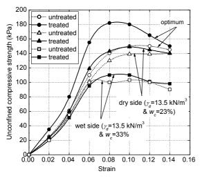
Figure 5. Effect of cutting stone slurry waste on the unconfined compressive strength for soil-2 at the optimum, dry, and wet sides of the optimum
