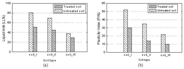
Figure 3. Effect of cutting stone slurry waste on: a) liquid limit and b) plasticity index of clayey soils
