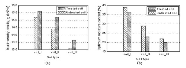
Figure 2. The effect of cutting stone slurry waste on: a) maximum dry density and b) optimum water content
