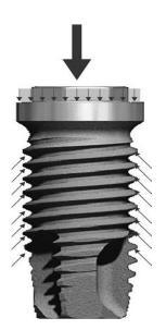
**Figure 2** Axial load distribution. The morphology of the threads can have an influence on the nature of compressive force created within the bone around a machined implant (figure adapted from Palacci et al. 1995)
