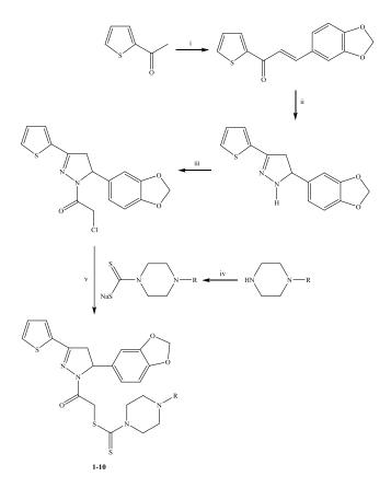
Scheme 1. The synthetic route for the preparation of new pyrazoline derivatives (1-10). Reagents and conditions: (i) Piperonal, 10% aqueous sodium hydroxide solution, ethanol, rt, 6 h; (ii) 80%  $NH_2NH_2.H_2O$ , ethanol, reflux, 3 h; (iii) ClCOCH<sub>2</sub>Cl, TEA, dry acetone, rt, 2 h; (iv) CS<sub>2</sub>, NaOH, rt, 1 h; (v) Acetone, rt, 3 h.
