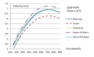
**Figure 14** Velocity calculated with different formulas versus discharge rate for  $\phi$ 200 HDPE pipe having slope 1/7
