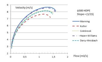
**Figure 12** Velocity calculated with different formulas versus discharge for  $\phi$ 500 HDPE pipe having slope 1/15
