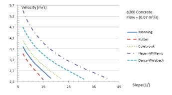
Figure 18 Velocity calculated with different formulas versus slope for  $\phi$ 200 concrete pipe having flow of 0.07 m<sup>3</sup>/s
