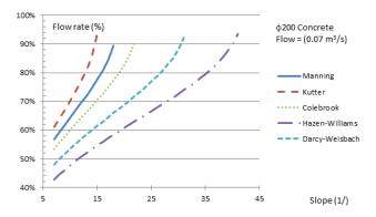
**Figure 16** Discharge rate calculated with different formulas versus slope for  $\phi$ 200 concrete pipe having flow 0.07 m<sup>3</sup>/s
