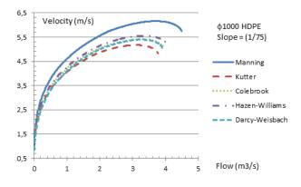
**Figure 13** Velocity calculated with different formulas versus discharge for  $\phi$ 1000 HDPE pipe having slope 1/75
