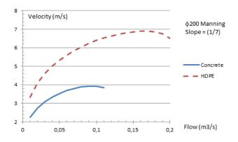
Figure 3 Velocity calculated with Manning formula versus discharge of the pipe of  $\varphi 200$  with slope 1/7
