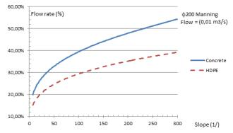
**Figure 5** Discharge rate (velocity calculated with Manning formula) versus slope of the pipe of  $\phi$ 200 having discharge of 0,01 m<sup>3</sup>/s
