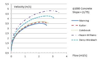
**Figure 8** Velocity calculated with different formulas versus discharge for  $\phi$ 1000 concrete pipe having slope 1/75
