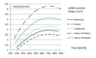
**Figure 9** Velocity calculated with different formulas versus discharge rate for \$200 concrete pipe having slope 1/7
