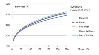
**Figure 17** Discharge rate calculated with different formulas versus slope for  $\phi$ 200 HDPE pipe having flow 0.01 m<sup>3</sup>/s
