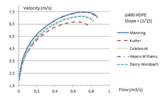
Figure 11 Velocity calculated with different formulas versus discharge for  $\phi 400$  HDPE pipe having slope 1/15
