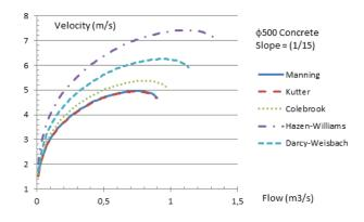
Figure 7 Velocity calculated with different formulas versus discharge for  $\phi$ 500 concrete pipe having slope 1/15
