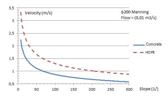
**Figure 4** Velocity calculated with Manning formula versus slope of the pipe of \$\phi200\$ having discharge of 0,01 m<sup>3</sup>/s
