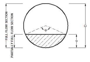
Figure 1 Hydraulic definitions of partially full flow [6]
