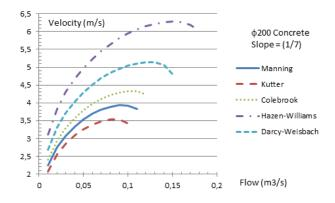
Figure 6 Velocity calculated with different formulas versus discharge for  $\phi 200$  concrete pipe having slope 1/7
