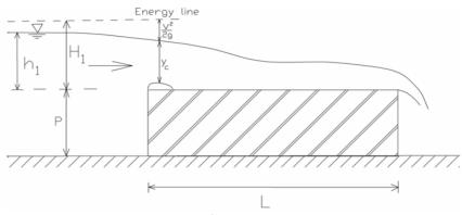
Figure 1-Flow pattern above a broad-crested weir
