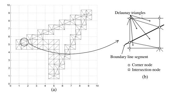
Figure 5. Test example; a) boundary line containing cells , b) nodes and Delaunay triangles for a chosen cell
