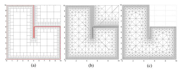
Figure 13. a) Quad-tree grid, b) triangulation based on quad-tree, c) mesh after post processing
