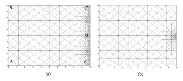
Figure 8. a) Type-I and b) Type-II triangular mesh
