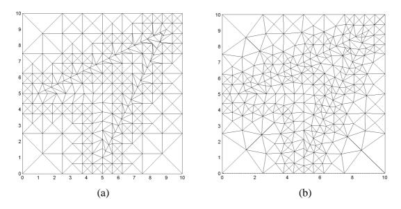
Figure 6. Test triangulation a) before and b) after Laplacian smoothing
