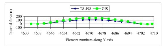
b) Maximum internal forces of the roof in Kalkandere
