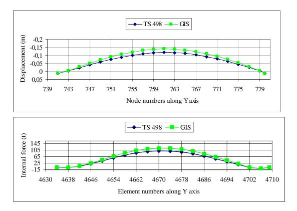
Fig. 10. Response of the sport hall roof under the snow loads in Rize
