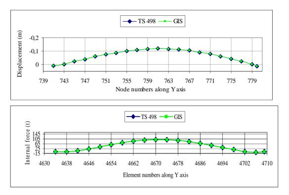
Fig. 9. Response of the sport hall roof under the snow loads in Trabzon
