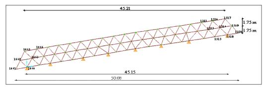
c) Plan of space roof truss in y-z plane
