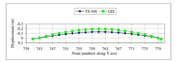
a) Maximum displacements of the roof in Kalkandere
