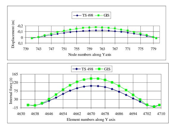
Fig. 11. Response of the sport hall roof under the snow loads in Artvin
