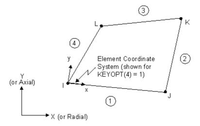
Fig. 2. Coupled-field solid element type (PLANE13)
