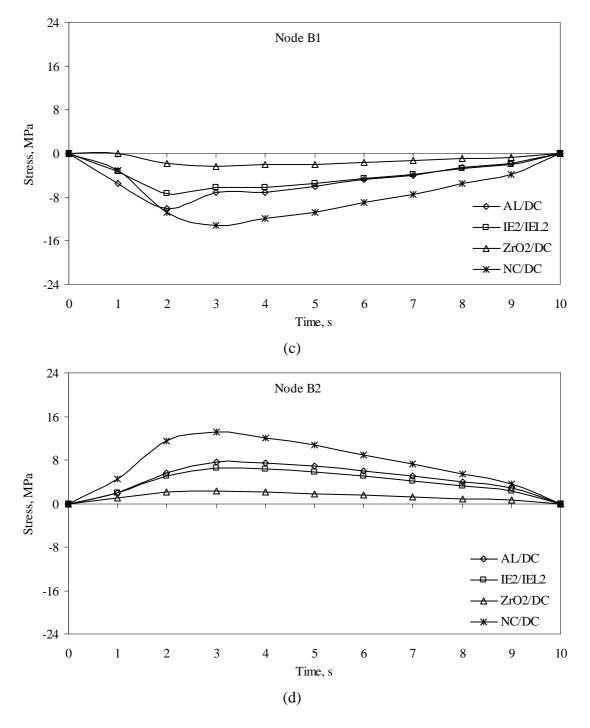
Fig. 6. Thermal stress distributions for x-direction at selected nodes by hot liquid
