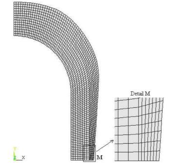
Fig. 3. The axisymmetric finite element model of the crown structure
