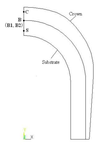
Fig. 1. The schematic geometry of model with considered nodes
