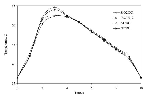
Fig. 4. Temperature changes depending on time at Node B caused by hot liquid
