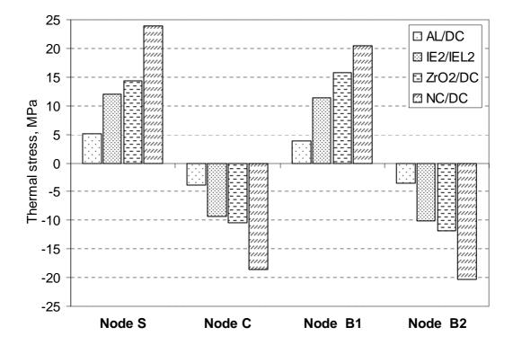
Fig. 9. The maximum values of thermal stresses at selected nodes caused cold liquid
