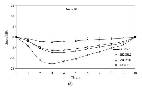
Fig. 7. Thermal stress distributions for x-direction at selected nodes by cold liquid
