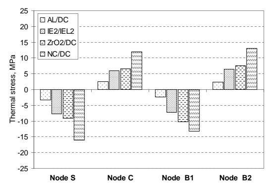
Fig. 8. The maximum values of thermal stresses at selected nodes caused hot liquid
