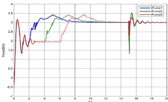
(a) Active power of three pair of wind turbine
