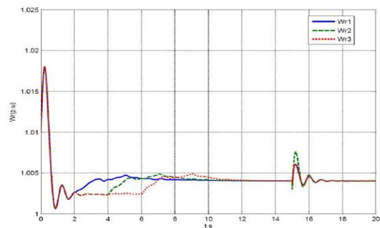
(b) Rotor speed of three pair of wind turbine
