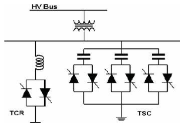
Fig. 2 Static Var Compensator (SVC)
