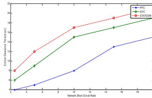
Fig. 11 Variation of critical clearance time with network SCR
