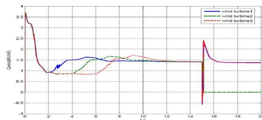
(b) Reactive power of three pair of wind turbine
