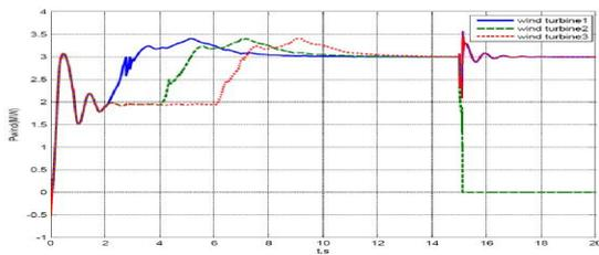
(a) Active power of three pair of wind turbine
