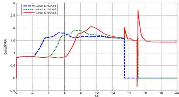
(b) Reactive power of three pair of wind turbine
