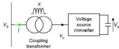
Fig. 1 STATCOM Configuration
