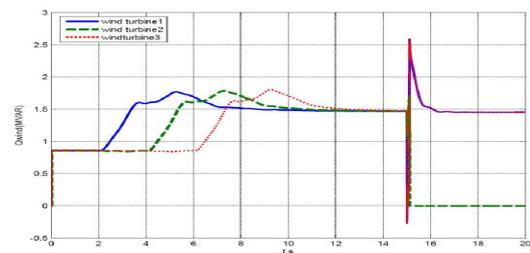
(b) Reactive power of three pair of wind turbine
