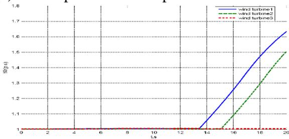
(c) Rotor speed of three pair of wind turbine
