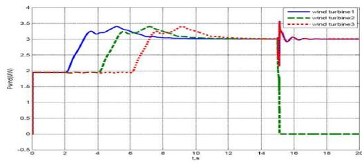
(a) Active power of three pair of wind turbine
