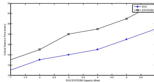
Fig. 12 Variation of critical clearance time with compensation device rating
