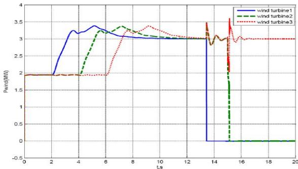
(a) Active power of three pair of wind turbine
