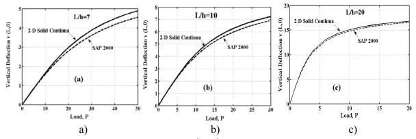
**Figure 5.** Load-vertical displacement (v(L,0)) curves for some given point loads and various ratios of lenght / height (L/h) for beam in the geometrically nonlinear case, a) L/h = 7, b) L/h = 10, c) L/h = 20, 2-D Solid Continua (-----); Sap 2000 (-----).
