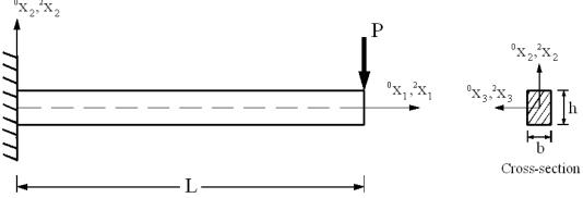
Figure 1. Cantilever beam subjected to a point load.
