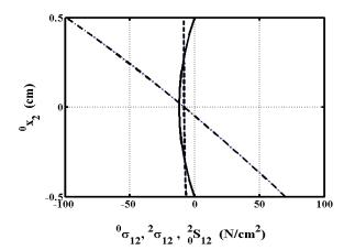
**Fig. 7.** Shear stresses of the cross section at the fixed end of the beam for P=8 N.  ${}^{0}\sigma_{12}(---); {}^{2}\sigma_{12}(----); {}^{2}_{0}S_{12}(---).$
