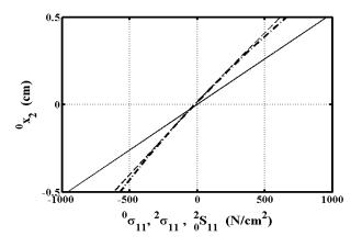
**Fig. 6.** Normal stresses of the cross section at the fixed end of the beam P=8 N.  ${}^{0}\sigma_{11}(---); {}^{2}\sigma_{11}(---); {}^{2}_{0}S_{11}(---).$
