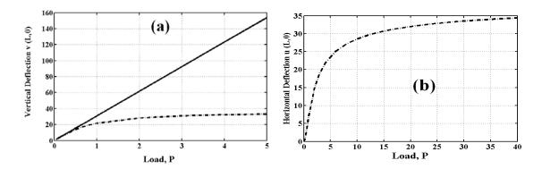
**Figure 4.** a) Load-vertical displacement (v(L,0)) b) Load- horizontal displacement (u(L,0)) curves for geometrically linear and geometrically nonlinear cases, Lineer (----); Nonlineer (----).
