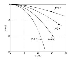
Figure 3. The displaced configuration of the axis of beam for some given point loads.
