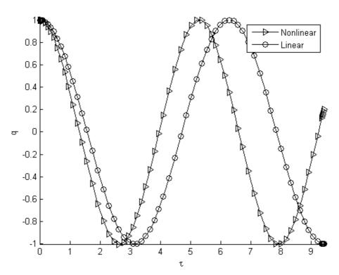
Fig. 4. Time history of dimensionless amplitudes for non-classical microscale beams
