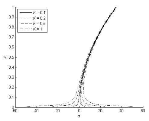
Fig 5. Effects of amplitude of excitation k for  $\gamma = 100$  in primary resonance.
