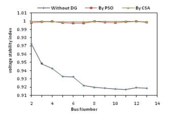
Figure 3. Voltage stability index of the case study network without and with three optimal DGs.
