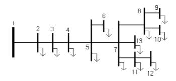
Fig. 3. Single line diagram of feeder.
