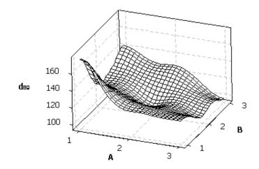
Fig.2. Response surface plots showing the effect of ball size (A) and fractional ball charge (B) on  $d_{80}$  size at level 2 of speed of rotation (C)
