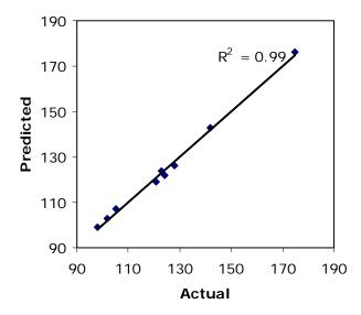
Fig.5.Predicted versus actual for d<sub>80</sub> size
