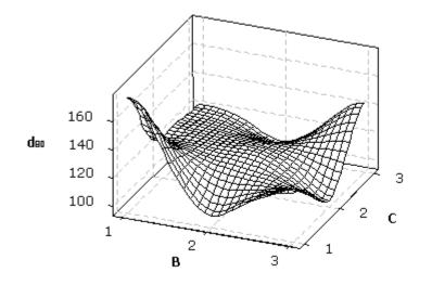
Fig.4. Response surface plots showing the effect of fractional ball charge (*B*) and speed of rotation (*C*) on  $d_{80}$  size at level 2 of ball size (*A*)
