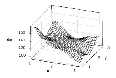
Fig.3. Response surface plots showing the effect of ball size (A) and speed of rotation (C) on  $d_{80}$  size at level 2 of fractional ball charge (B)
