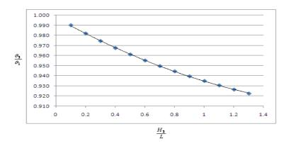
Fig.3. Ratio of efflux time for different values of  $H_2/L$  ( $D_1=D_2$ )
