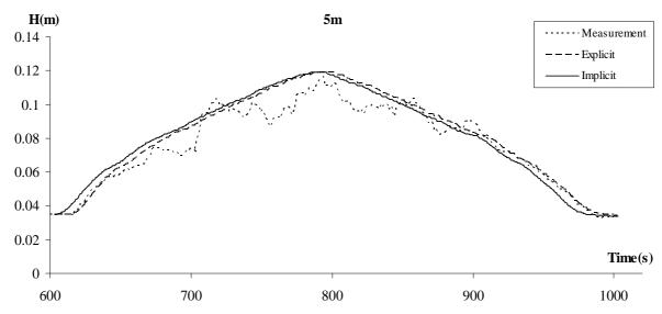
**Fig. 10a.** Comparison of flow depth for hydrograph 2 in x=5m
