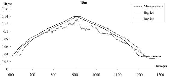
Fig. 8d. Experimental and numerical results for flow depth in x=15m and Hydrograph 1
