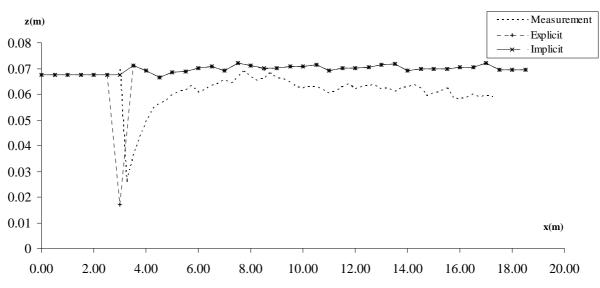
Fig. 9. Comparison of experimental and numerical results for bed profile in Hydrograph 1
