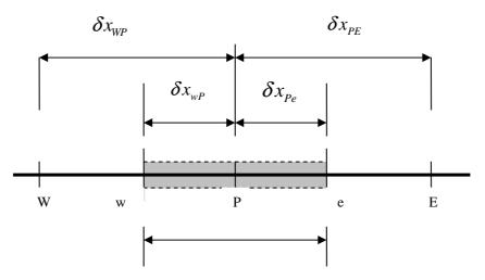
Fig. 2. Illustration of finite volume method in one dimensional
