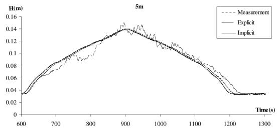
Fig. 8a. Experimental and numerical results for flow depth in x=5m and Hydrograph 1
