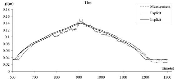
Fig. 8c. Experimental and numerical results for flow depth in x=11m and Hydrograph 1
