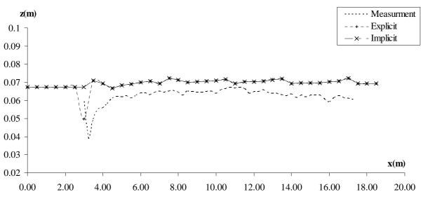
Fig. 11. Comparison of experimental and numerical results for bed profile in Hydrograph 2
