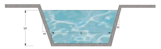
Fig. 3. Geometric dimensions of open canal with trapezoidal cross sections
