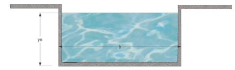
Fig. 2. Geometric dimensions of open canal with rectangular cross sections
