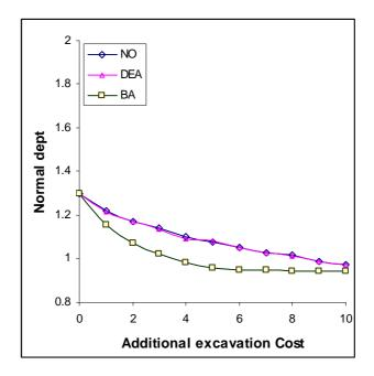
Fig. 5.Variation of optimum nondimensional side slope and normal depth of a triangular section with  $\beta_L = 1.0$
