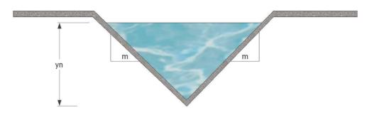
Fig. 1. Geometric dimensions of open canal with triangular cross sections
