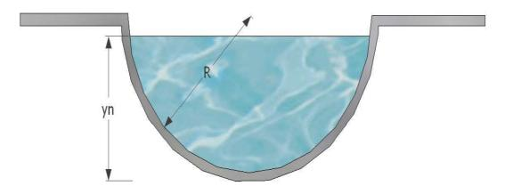
Fig. 4. Geometric dimensions of open canal with circular cross sections
