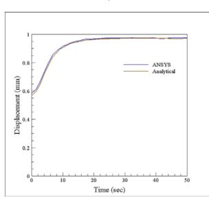
Figure 4. Comparison of effect of thermal and pressure loading on displacement for two methods
