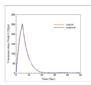
Figure 3. Comparison of effect of thermal and pressure loading on Von-mises at 8 nodes stress for two methods
