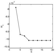
**Fig.2** Convergence of non-dimensional deflection of the plate at a location (R = 0.5) 5.3 Effect of material heterogeneity indices
