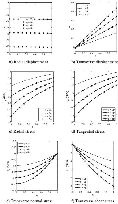
Fig.5 Effect of the loads ratio on physical quantities across the plate thickness
