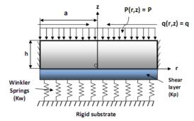
Fig. 1 Geometry of 2D-FGMs circular plate resting on elastic foundation
