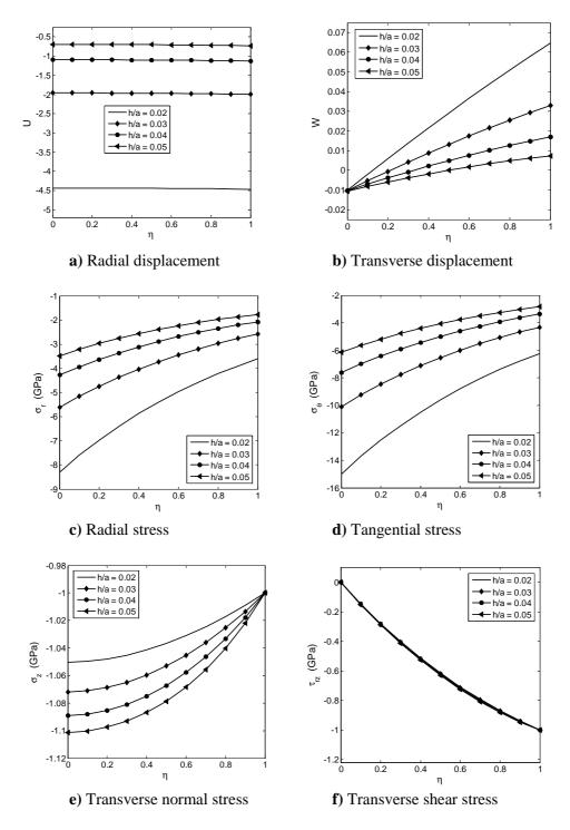
Fig.4 Effect of the geometric parameter (thickness to radius ratio) on physical quantities across the plate thickness
