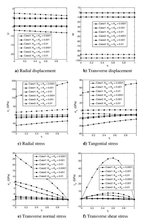
Fig.6 Effect of the foundation stiffnesses coefficients on physical quantities across the plate thickness
