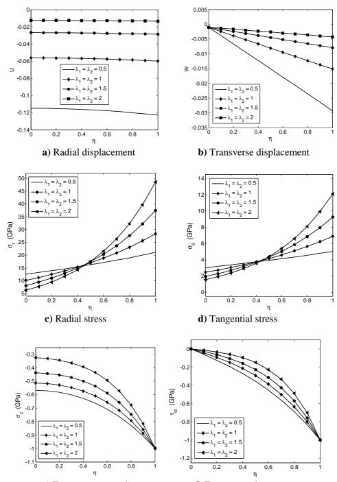
e) Transverse normal stressf) Transverse shear stressFig.3 Effect of the material heterogeneity indices on physical quantities across the plate thickness
