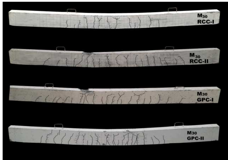
Figure 8: Crack Pattern of RCC and GPC Beams
