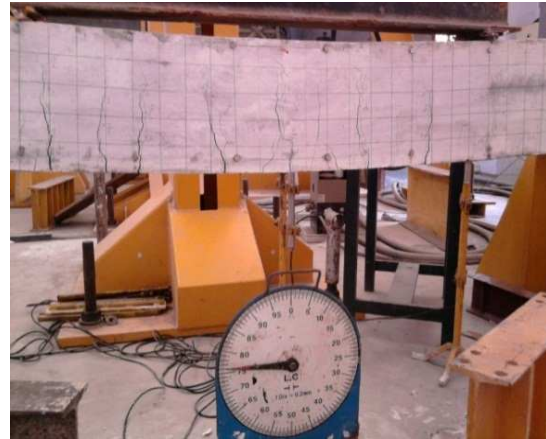
Figure 6: Crack Pattern Control Beam
