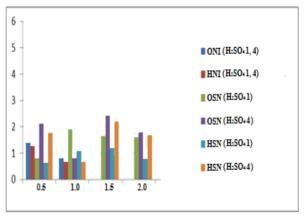
Figure 8. Percentage of loss of water by H<sub>2</sub>SO<sub>4</sub> 1 and 4 Percentage
