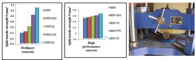
Figure 5. Split tensile strength of concrete specimens
