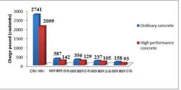
Figure 9. Rapid Chloride Permeability Test results
