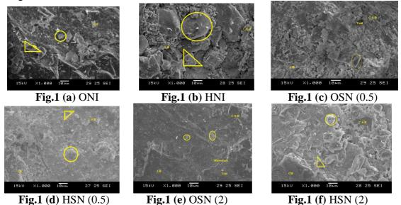
Figure 1 SEM results of ordinary and high performance concrete without and with inhibitor
