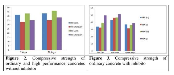
The compressive strength of cubes and cylinders of ordinary concrete with inhibitor at 7 days and at 28 days is shown in Fig.3. The compressive strength of cubes and cylinders of high performance concrete with inhibitor at 7 days and at 28 days and the test setup are shown in Fig.4.
