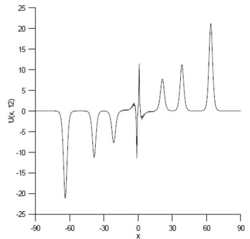
**Figure 3:** Simulation of the clash of two solitary waves
