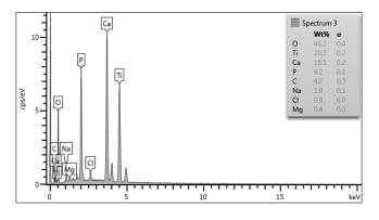
Figure 5.EDS analysis results for coating surfaces obtained
