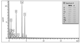
**Figure 6.**EDS analysis results for coating surfaces obtained by waiting for 96 hours in SBF
