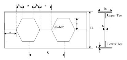
Fig. 2. Geometry and notation for cstellated beam
