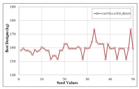
Fig. 7. Effect of Seed Values for 5-m span beam with 500 iterations
