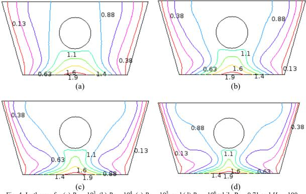
Fig. 4: Isotherms for (a)  $Ra = 10^3$ ; (b)  $Ra = 10^4$ ; (c)  $Ra = 10^5$ ; and (d)  $Ra = 10^6$  while Pr = 0.71 and Ha = 100
