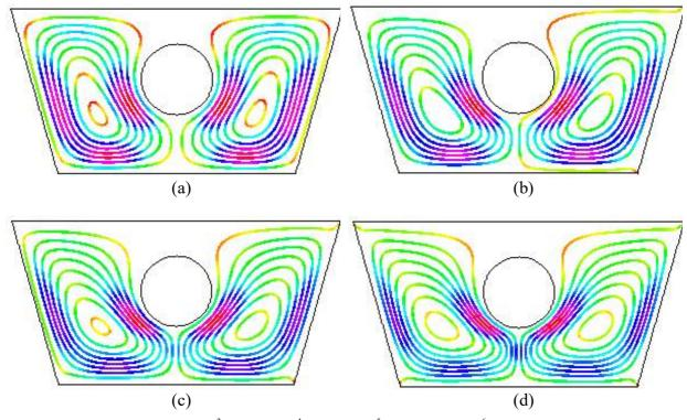
Fig. 3: Streamlines for (a)  $Ra = 10^3$ ; (b)  $Ra = 10^4$ ; (c)  $Ra = 10^5$ ; and (d)  $Ra = 10^6$  while Pr = 0.71 and Ha = 100
