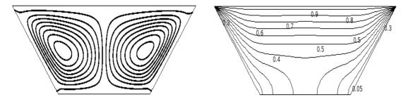
Fig. 2(b): Obtained results of streamlines and isotherms by present work
