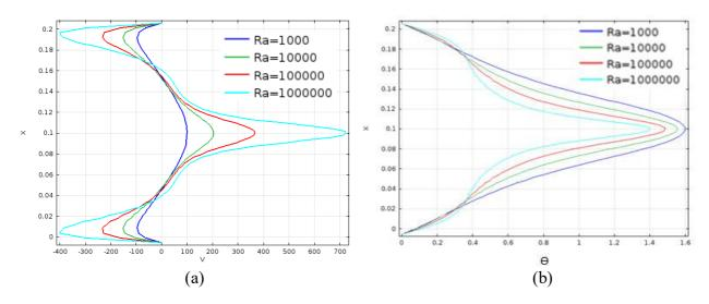
Fig. 5: (a) Velocity profiles and (b) Temperature profiles for Hartmann number Ha = 100 and Pr = 0.71 with varying Rayleigh number  $Ra = 10^3 - 10^6$  along the bottom wall
