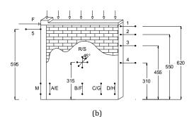
Figure 2. (a) Wall model and apparatus; (b) dimensions and point of measure
