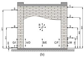
Figure 3. (a) Apparatus of cyclic tests; (b) points of measure of wall.
