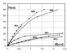
Figure 4. Experimental horizontal force vs displacement at the top of walls
