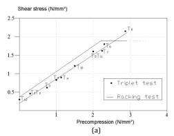
Figure 6. Comparison of triplet results with racking tests results
