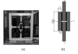
Figure 1. (a) Experimental apparatus; (b) triplet specimen
