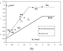
Figure 7. Comparison of exp. results on shear walls with EC6 criterion.
