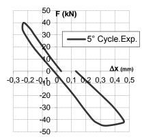
Figure 5. Cyclic experimental diagram at 5<sup>th</sup> cycle of loading (C1)
