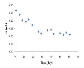
Fig. 9 Storage stability of the biosensor (0.05 M, pH 9.5 borate buffer at 0.3 V).
