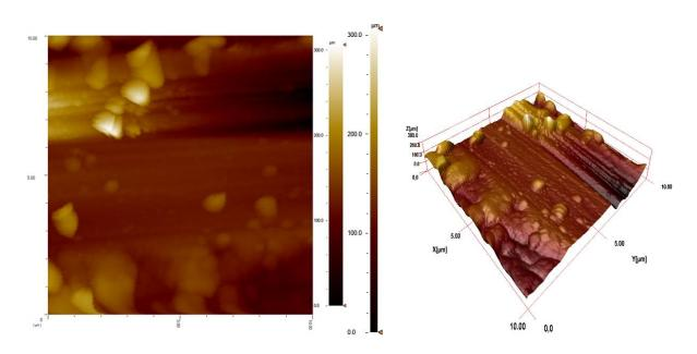
Fig.2 AFM images of (a) Pt/PPy-pTS electrode and (b) Pt/PPy-pTS-uricase electrode
