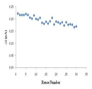
Fig. 8 The reusability performance of the biosensor  $(0.05 \text{ M}, \text{pH } 9.5 \text{ borate buffer at } 25^{\circ}\text{C}).$
