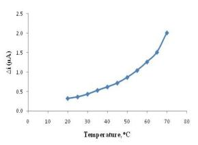
Fig. 4 Effect of temperature on the current response of the biosensor (at 0.3 V in  $5.0 \times 10^{-5} \text{ M}$  uric acid solution of borate buffer, pH 9.5).
