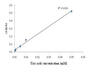
Fig. 6 The calibration curve of the uric acid biosensor (in pH 9.5 borate buffer at 0.3 V).
