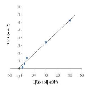
Fig. 7 The effect of uric acid concentration on the amperometric response of the biosensor (Lineweaver-Burk plot, in pH 9.5 borate buffer at 0.3 V).
