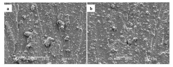
Fig.1 SEM images of (a) Pt/PPy-pTS electrode and (b) Pt/PPy-pTS-uricase electrode
