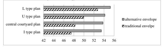
Fig. 17. The comparison of cooling load for traditional and alternative building envelope with the same U-value for reference building (A/V=0.5).
