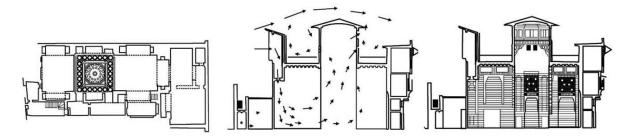
Fig. 5. Plan and section of the hall of Muhib Ad-Din Ash-Shaf'i AI-Muwaqqi, Cairo, Egypt, showing how the malqaf produce air movement internally. Arrows indicate the direction of airflow; arrow length corresponds to airspeed [19].
