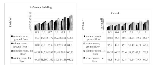
Fig. 16. Comparison of cooling load for seasonal rooms, I type plan.
