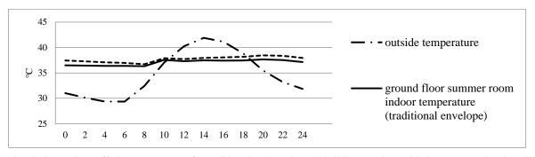
Fig.18. Comparison of indoor temperature for traditional and mostly used building envelope with the same U-value On July 21(I type reference building, A/V=0.50).
