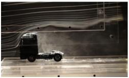
Fig.9. Flow visualization of truck
