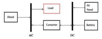
Fig.1. The block diagram of PV/diesel hybrid power system
