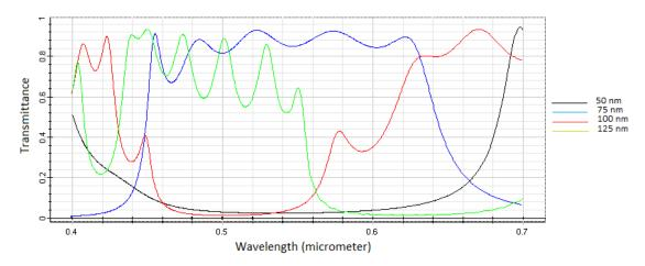
Figure 3. Transmittance of  $TE_{\nu}$  which layer thicknesses are 50 nm, 75 nm, 100 nm, 125 nm
