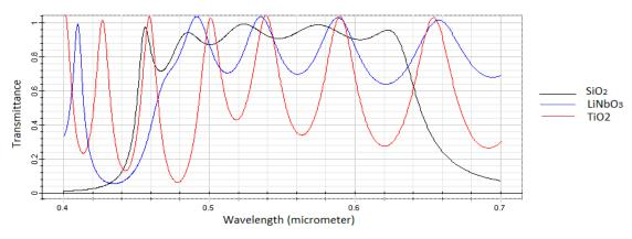
**Figure 5.** Transmittance graph of  $TE_y$  in  $SiO_2 - W$ ,  $LiNbO_3 - W$  and  $TiO_2 - W$
