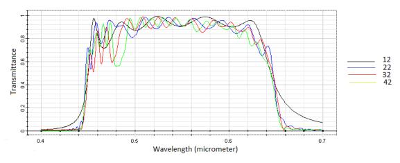
Figure 4. Transmittance graph of  $TE_{y}$  which layer number is 12, 22, 32 and 42
