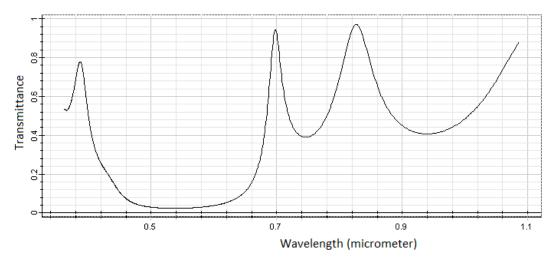
Figure 2.  $TE_y$  transmittance of 1D MDPC
