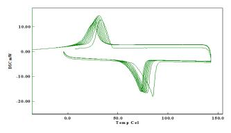
Fig. 4. The thermal cycles of DSC curves of heat treated sample at 800 C.
