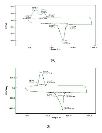
Fig. 1. Schematic illustration of DSC result for a) as-cast and b) heat treated at 800 °C sample.
