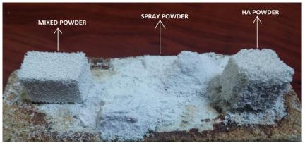
Figure 5. Preforms of different situations powder morphology
