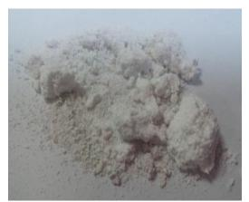
Figure 4. The collapsed HA foam produced from spray dried powder after sintering
