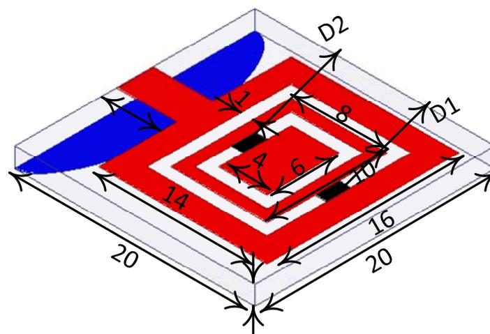
**Fig.1** configuration of antenna structure
