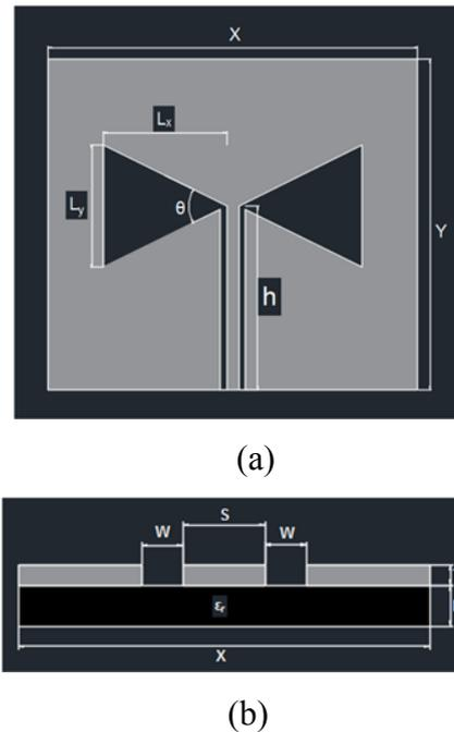
**Figure 3.** The geometric structure of the proposed antenna. **(a)** Top view. **(b)** Side view.
