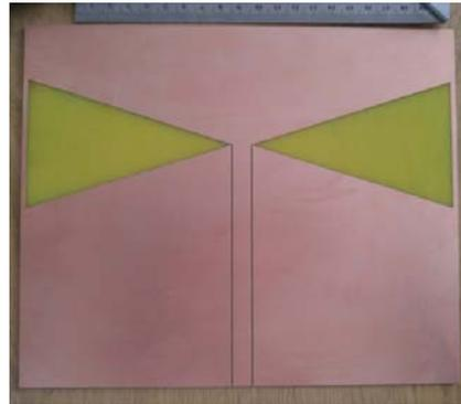
**Figure 7.** Photograph of fabricated Bow tie Antenna
