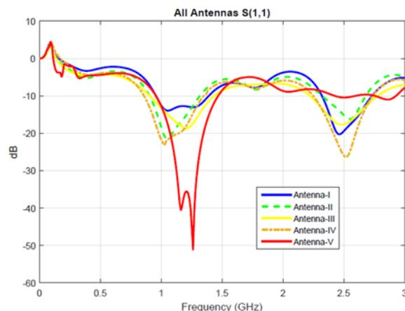
**Figure 4.** S11 graphs of simulated antenna.
